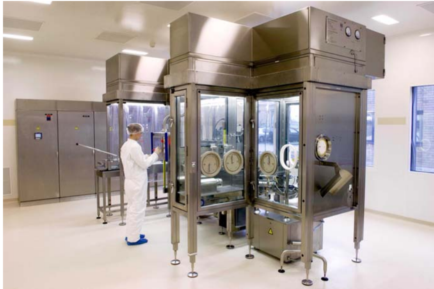
Figure 2 - Restricted Access Barrier System (RABS) encloses a vial filling line, and helps to ensure the aseptic environment (courtesy of Telstar North America)
