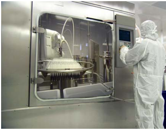
Figure 1 – Aseptic isolator with a Stäubli Stericlean, six-axis robot arm that is compatible with vapor phase hydrogen peroxide sterilization (courtesy of Stäubli Robotics)
