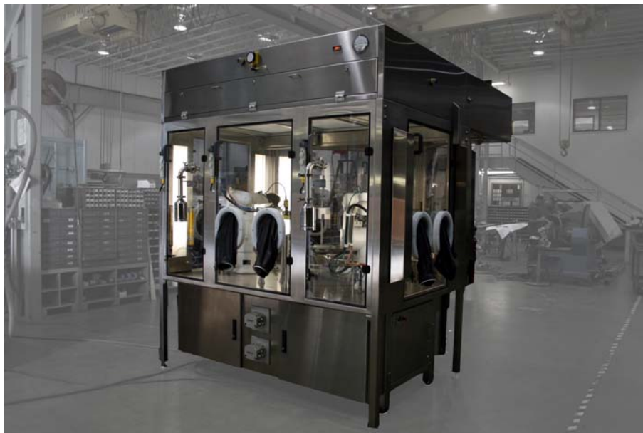
Figure 4 – ANSI/RIA R15.06-1999 robot safety compliant RABS unit that protects the operator from the robot system and protects the product from contamination originating from the operator (courtesy of Automated Systems of Tacoma)
